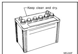
When the vehicle is not going to be used over a long period of time, disconnect the battery cable from the negative terminal.
