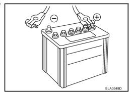
Check the charge condition of the battery.
